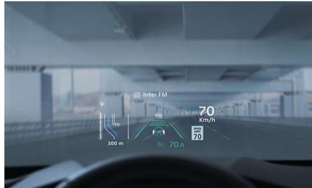
Projected directly on the windshield, the available 10.8" full-colour Head-Up Display relays the most relevant driving information (speed, navigation, advance safety features) directly in your line-of-sight, resulting in greater focus on the road and overall safety.
