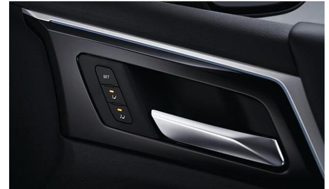
The available 8-way Power Driver's Seat with memory is linked to the FAST-Key fobs, so the optimal seat and side-view mirror positions for each driver can be personalized and saved. The available 4-way Power Front Passenger Seat with memory adds additional convenience so the passengers can also save their preferred seat position.
