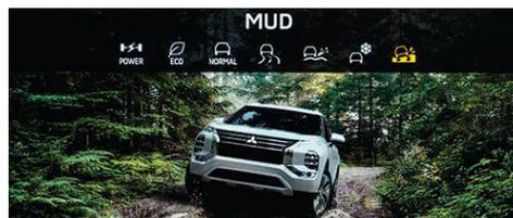
**MUD** enhances performance when driving through muddy or deep snow conditions, especially when accelerating and/or turning from a stopped position.
