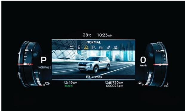
The 12.3" full Digital Driver Display provides all the important driving and safety information you need in high-resolution, including speed, navigation, safety data, S-AWC settings, battery state-of-charge, total range, EV modes and much more.
